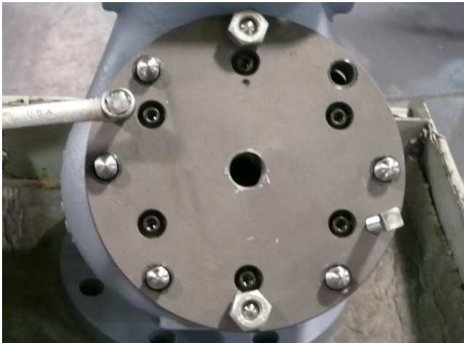
Figure 10-1 Alternately Tighten Jack Screw
