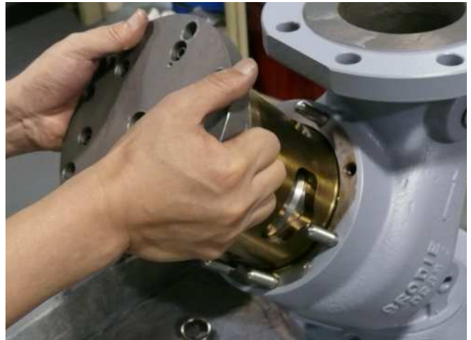
Figure 10-2 Remove Cylinder Assembly From Valve Body
