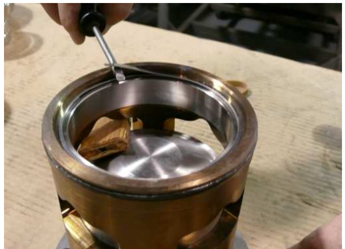
Figure 10-4 Spirolox Retaining Ring
