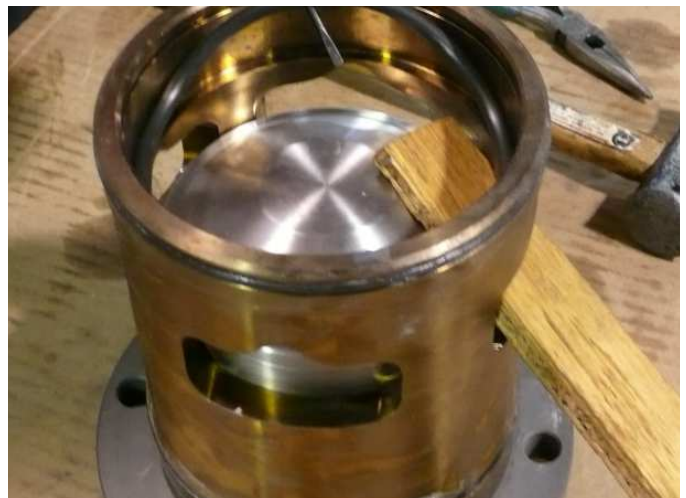
Figure 10-3 Block Piston In Open Position
