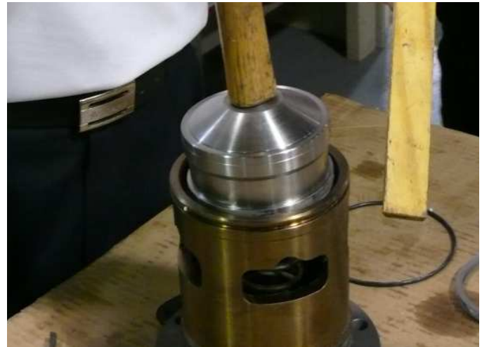
Figure 10-7 Removing Spring From Cylinder
